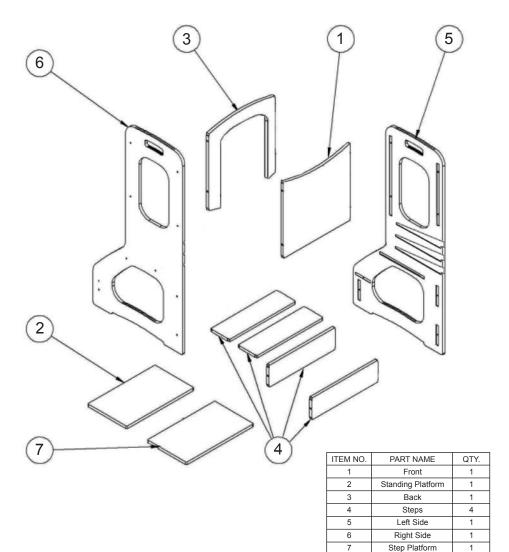
Insert pieces into allocated slots as pictured Fix in place using a screwdriver.
